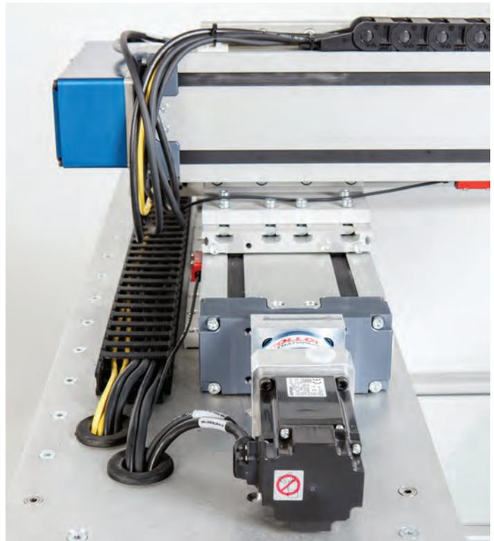
Box incorporates Rollon's TH series (TH 110 and TH 145) linear actuators. These compact, pre-loaded, ball-screw-driven units have zero backlash and offer positioning accuracy and repeatability within 5  $\mu\text{m}$ .
